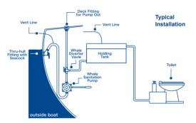
Note: Where discharge is below the water line, a siphon break must be fitted.
