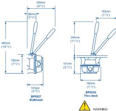
It is important to ensure that a syphon break is fitted, where discharge is below the water line.
