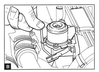
Pump the supply pump (B) with the lever until air free fuel comes out of the bleed screw. Tighten the bleed screw on the filter. If the supply pump drive cam is in position for maximum cam lift it is not possible to pump by hand. In this situation the crankshaft must be turned one revolution.
