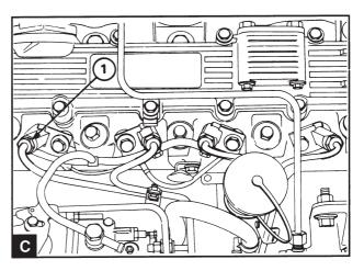
Slacken off the connector nuts for the delivery lines at the injectors (C). Depending on the type of injectors the connector nuts can be located above or beside the injectors.
