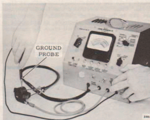
Figure 4-10. Coil Leakage Test
