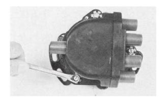
**46.** Remove the distributor cap, 3 screws. Tool width: 8 mm.
