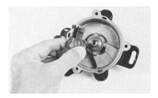
**47.** Remove and replace the rotor. Re-install the distributor cap.
