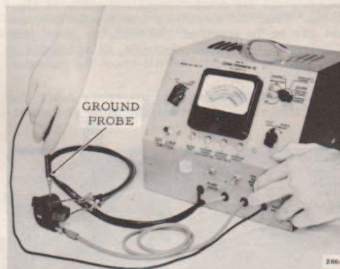
Figure 4-10. Coil Leakage Test
