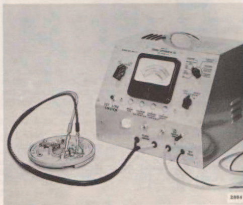
Figure 4-12. Breaker Point Testing
