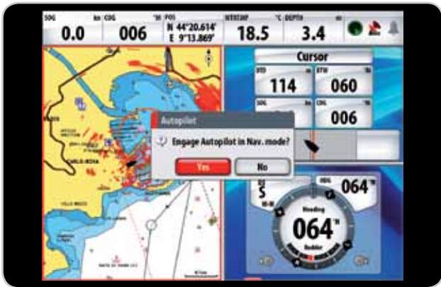
NSE RTM2.0 Software prompting whether you want to engage the Autopilot in Nav mode
