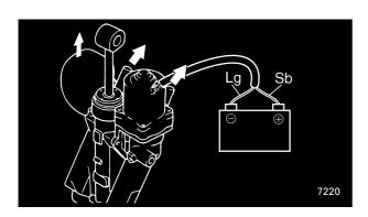
(3) Connect the leads on the battery terminals in the up position until the trim and tilt ram assemblies are fully extended.
